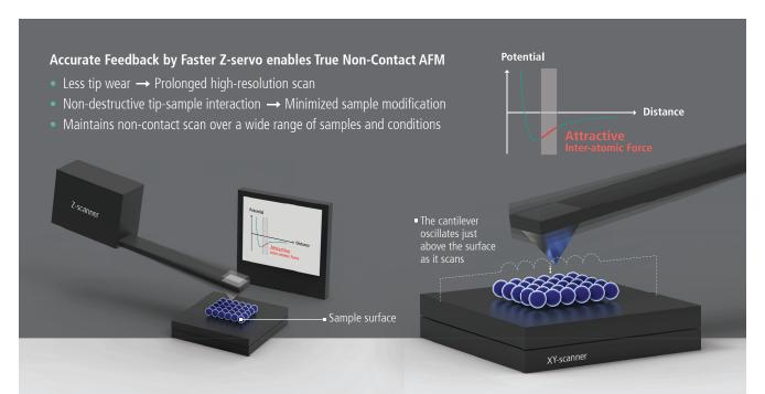
Unlike in contact mode, where the tip contacts the sample continuously during a scan, or in tapping mode, where the tip touches the sample periodically, a tip used in non-contact mode does not touch the sample.
