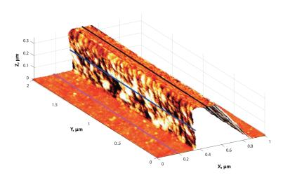
3D AFM image provide high resolution profiles for bottom, sidewall, and top of the photoresist line, which can be used for LER/sidewall roughness analysis of the structure
