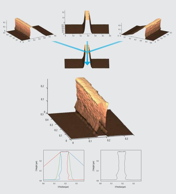
■ Images taken at three different tilting angles can be stitched to combined together automatically to form a complete 3D image
