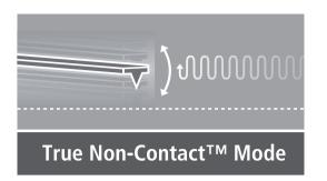
In this technique, the cantilever oscillates just above the surface as it scans. A precise, high-speed feedback loop prevents the cantilever tip from crashing into the surface, keeping the tip sharp and leaving the surface untouched. As the tip approaches the sample surface, the oscillation amplitude of the cantilever decreases. By using the feedback loop to correct for these amplitude deviations, one can generate an image of the surface topography.
