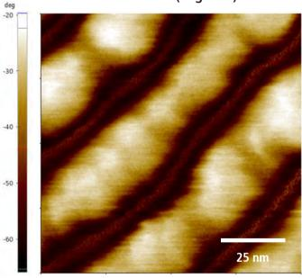
System: Park NX10 Scan Mode: Tapping Scan Size: 0.5µm × 0.5 µm Image Resolution: 256 px  $\times$  256 px
