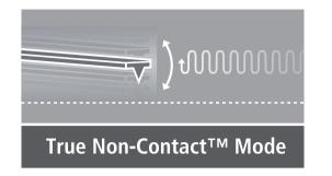
In this technique, the cantilever oscillates just above the surface as it scans. A precise, high-speed feedback loop prevents the cantilever tip from crashing into the surface, keeping the tip sharp and leaving the surface untouched. As the tip approaches the sample surface, the oscillation amplitude of the cantilever decreases. By using the feedback loop to correct for these amplitude deviations, one can generate an image of the surface topography.
