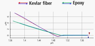
F/D mapping Conditions Mapping Size: 6 µm x 7 µm Mapping Points: 64 x 64 F/D Curve Pixels: 1,024 Force Limit: 6 V Approach Speed: 1 µm/s Retract Speed: 1 µm/s
