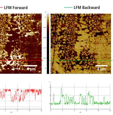
System: Park NX10 Scan Mode: LFM Scan Size: 20 µm x 20 µm Image Resolution: 512 px x 512 px
