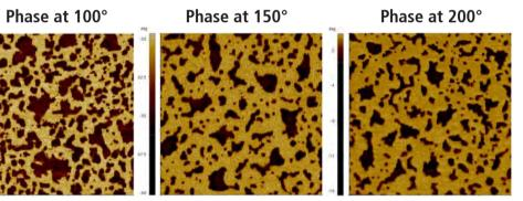
System: Park NX10 Scan Mode: Tapping, TCS2 Scan Size: 5 µm x 5 µm Image Resolution: 512 px x 256 px
