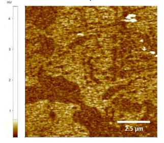
System: Park NX10 Scan Mode: PFM (vertical signal) Scan Size: 10µm×10µm Image Resolution: 256 px x 256 px Sample Bias: 0 V (DC) Tip Bias: 2 V (AC)
