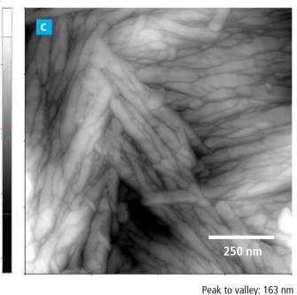
System: Park NX10 Scan Mode: Non-contact Scan Size:  $3 \mu m \times 3 \mu m$ ,  $5 \mu m \times 5 \mu m$ Image Resolution: 512 px x 256 px, 512 px x 256 px
