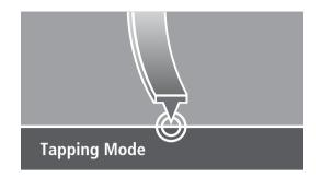
In this imaging mode, the cantilever also oscillates (as in non-contact mode) with the probe coming into intermittent contact with the sample surface. This enables improved imaging capability for certain samples whose surfaces require this type of interaction for optimal characterization (e.g., block copolymers).
