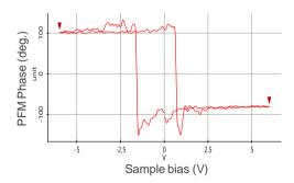
System: Park NX10 Scan Mode: PFM (lateral signal) Scan Size: 3 µm x 3 µm Image Resolution: 256 px x 256 px Sample Bias: 10 V (DC) Tip Bias: 1 V (AC)
