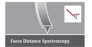
A force-distance curve is acquired by bringing the cantilever tip into contact with the sample surface. The shapes of specific regions of force-distance curves offer insight into different mechanical properties, such as adhesion, Young's modulus, etc.
