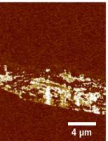
System: Park NX10 Scan Mode: PinPoint CP-AFM Scan Size: 20 µm x 20 µm Image Resolution: 256 px x 256 px Sample Bias: 10 V
