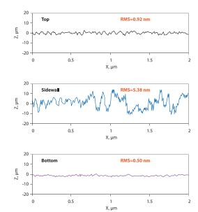
3D AFM image provide high resolution profiles for bottom, sidewall, and top of the photoresist line, which can be used for LER/sidewall roughness analysis of the structure
