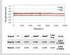
tact mode has several key advantages. Scanning at the highest resolution throughout imaging is now possible as the tip's sharpness is maintained. Non-contact mode avoids damaging soft samples as the tip and sample surface avoid direct contact.
