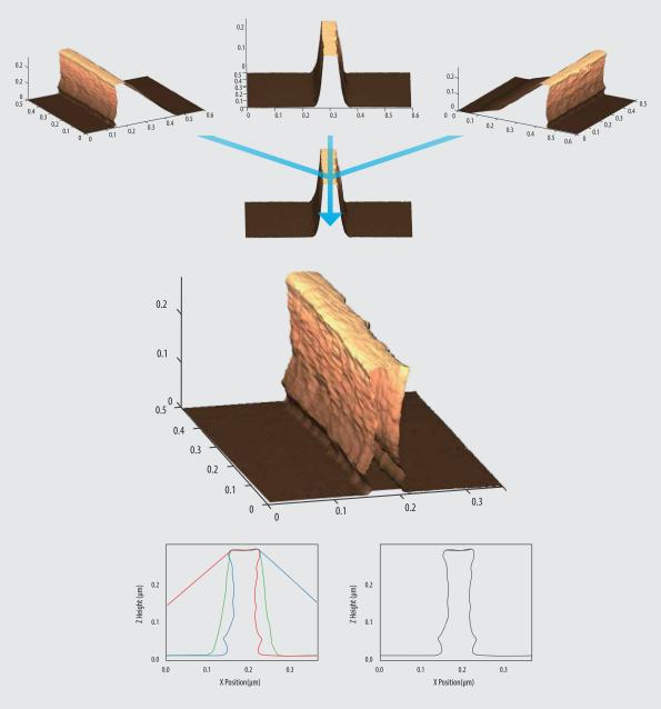
Images taken at three different tilting angles can be stitched to combined together automatically to form a complete 3D image
