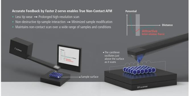
Unlike in contact mode, where the tip contacts the sample continuously during a scan, or in tapping mode, where the tip touches the sample periodically, a tip used in non-contact mode does not touch the sample. Because of this, use of non-con-
