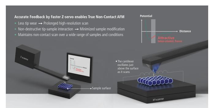
Unlike in contact mode, where the tip contacts the sample continuously during a scan, or in tapping mode, where the tip touches the sample periodically, a tip used in non-contact mode does not touch the sample.
